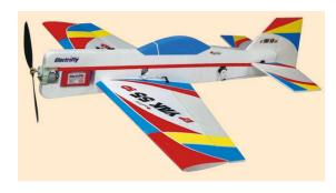
The Great Planes Yak 55 is a foamie profile plane. I picked it up at Airborne Hobbies for \$40, it comes with a nice brushed motor and gear box, carbon fiber wing and fuselage rods and air foiled wings. The plane has a full flying elevator. The kit even comes with servo arm extensions; you glue them onto your standard servo arm to give greater throw.
